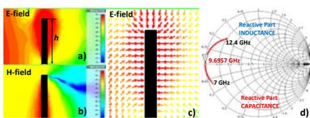
Waveguide discontinuities are illustrated on the example of waveguide rectangular (WR) in the manner like shown on your left for resonance post. Smith chart clearly demonstrates the series resonance and almost total energy reflection from the post.
