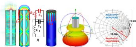
will understand how to manage them and build high-quality equivalent circuits required for fruitful computer simulation and optimization. You will accustom to reveal the frequency behavior of discontinuities through the curves on Smith charts like shown here for open-ended coax. Pay attention to a colorful image of
