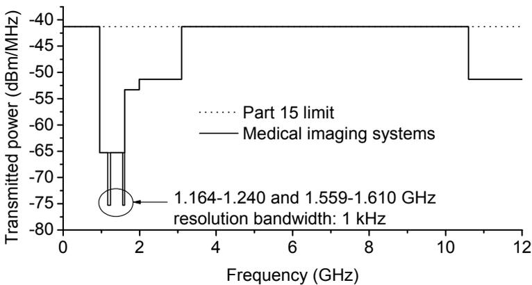
Fig. 47. FCC emission mask, medical imaging.
