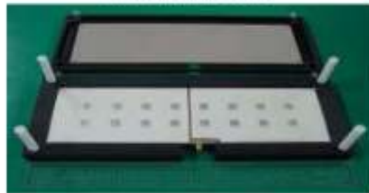
(b) Disassembled antenna structure
